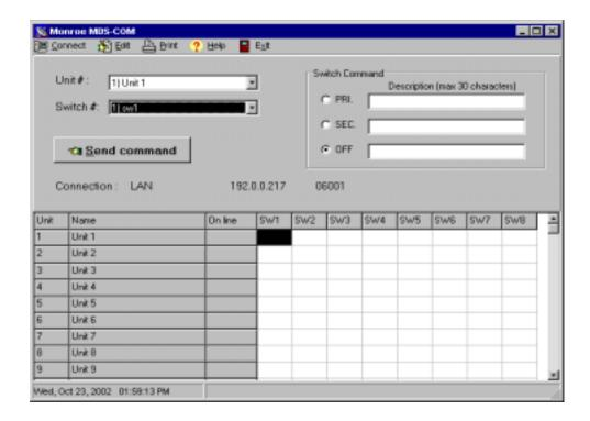
Upon entering the program, a table is displayed to show all 64 units each units switch status. After a switch command is sent and an O.K. message is received, the table will be updated. The status will be saved upon exiting the program, and read when opening the program.
